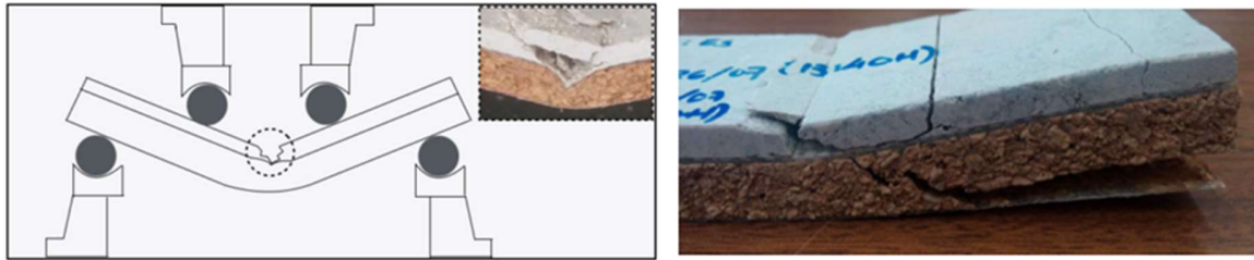
Figure 2.6 Left: Failure of specimen in 4-point bending (Gomes 2016). Right: Failure of specimen in cyclic 4-point bending
