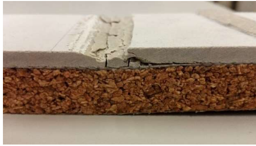
Figure 5.13 Failure for stone crushing after 30'000 cycles of L2C1 tested at 60% F_{UF}
