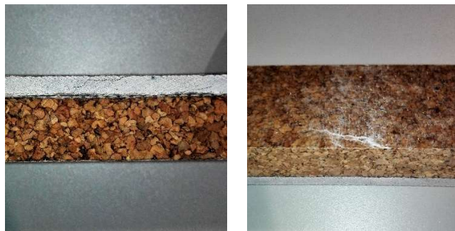
Figure 5.17 Specimen tested at 60% with resting time. Left: crack on the stone. Right: whitening of the resin.
