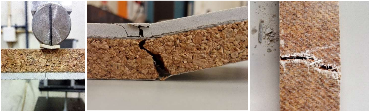
Figure 5.14 Failure modes observed for load percentage 55% (L2C1). Left: fracture of the limestone (the picture was taken in "reversed configuration" applying a tensional load on the stone to open the crack, for it to be easily seen. Center: fracture nucleated on the lower fibers. Right: picture of the fractured fibers.
